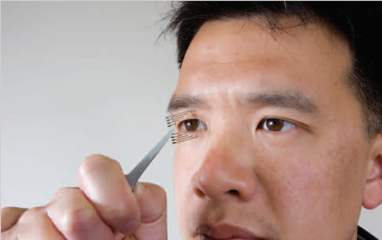
Dr. Chang peers through one of his tiny creations. A series of electrodes on a glass substrate, this chip is designed for growing cell axons. The image (above right) shows an axon he has coaxed to grow between two electrodes (shaded in black). He will use this and many other axons to test nanosurgical techniques.
